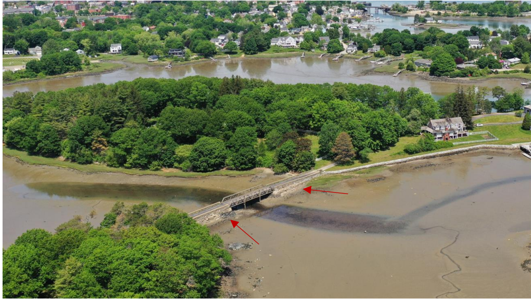
Figure 1: Scouring caused by existing tidal restriction – area to be restored.
