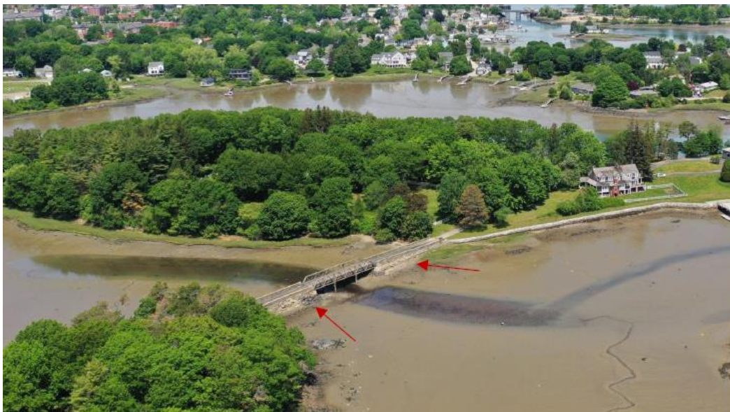
Figure 1: Existing tidal restriction to be eliminated and scoured area to be restored to mud flat.
